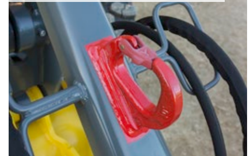
Load hook on the tilt rod (standard)
